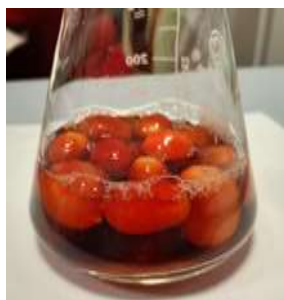
Photo No. 4-6 The process of formation of a chitosan film on the surface of tomato fruits.
