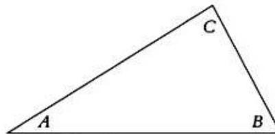
$$\angle A + \angle B + \angle C = 180^\circ$$
